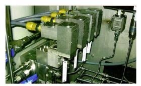
Inrada Oil & Gas systems include a hydraulic power unit which drives the actuated valves. The power units have a standard industrial design that can be installed in a safe area or engineered according to client specifications for installation in a zone 1 or zone 2 area. The hydraulic pump controls and starters are incorporated in the package to provide a plug & play solution.
